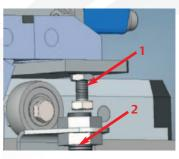
shapes are used, the position must be checked for all spool types. Set a distance of 0.5 to 1.0 mm between sensor (2) and actuator (1). The sensor has a LED that indicates an actuation.
