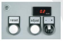
al, a negative value indicates a lower coil height than at the reference point. Actuate the "adjust" pushbutton switch to display the set permitted height deviation.
