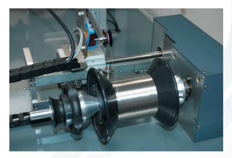
The sensor detecting the flange is mounted on the traversing system. At a defined point, the current distance is captured and saved as reference distance for each single layer. While the traversing system moves, the reference distance is continuously compared to the measured value.
